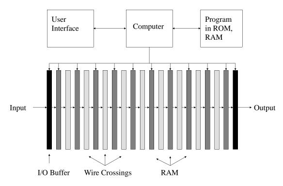
Figure VII.C. Hardware Implementation of MPJ
