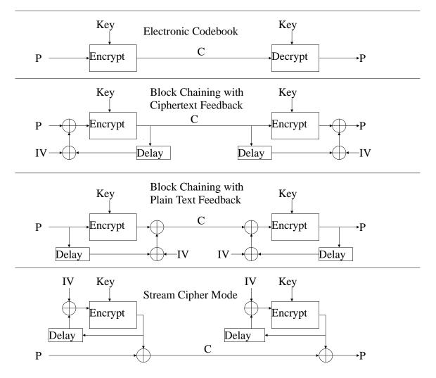
Figure III.D. Block Cipher Modes.
