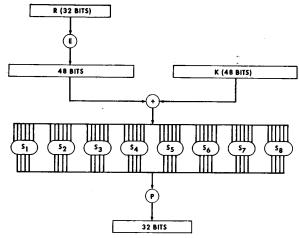
Figure V.H.2. DES Nonlinear Function
